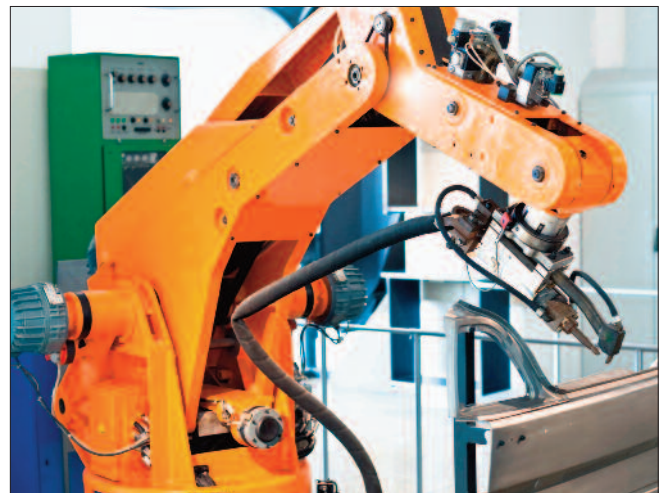
The simplest implementation of lights-out manufacturing is the replacement of a human arm with a robotic arm.
